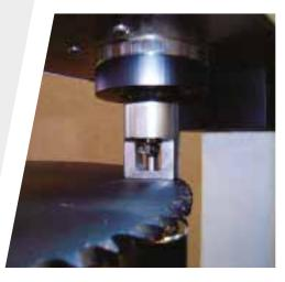
**Clamping Device** Removable clamping device supports oversize or odd shaped parts!
