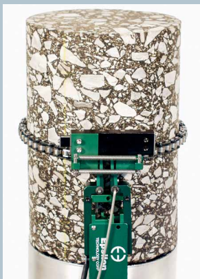
Model 3544-0400 with 1.25 inch to 4 inch diameter range
