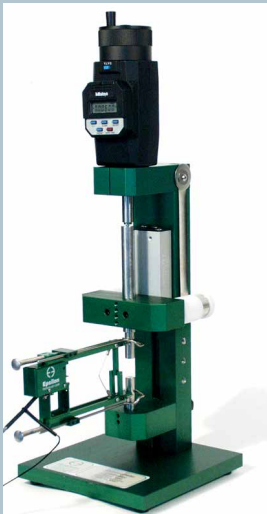
Model 3590 calibrator with Model 3542 axial extensometer
