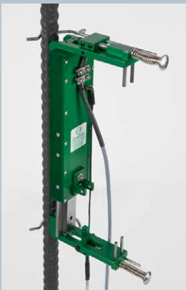
Model 3543 with 100 mm gauge length
