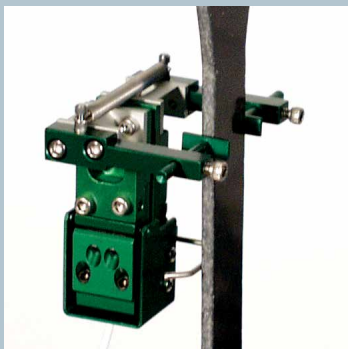
Model 3475-050T-ST with \pm 0.050 inch measuring range
