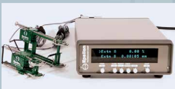
Model DSM-Plus two channel high accuracy strain meter with two Model 3542s
