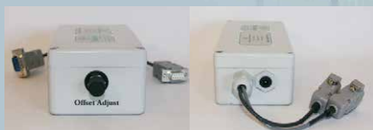
Model SGA single channel signal conditioner
