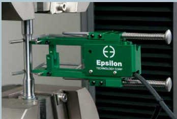
Model 3542 with 25 mm gauge length
