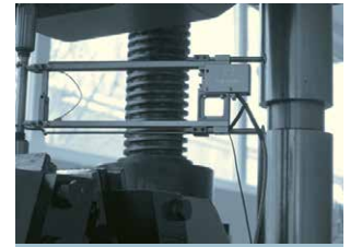
Model 3542 axial extensometer mounted on round tensile sample.
