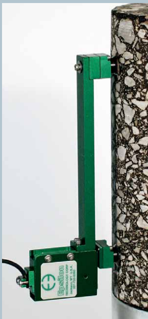
Model 3909-0400 with 4 inch gauge length
