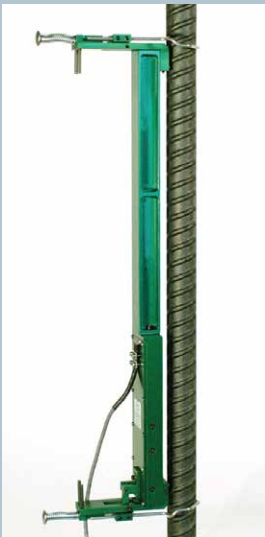
Model 3543 with 12 inch gauge length
