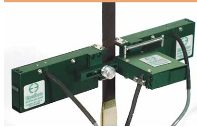
Model 3560 with 25 mm gauge length
