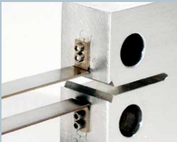
Model 3541 attached to bolt-on knife edges
