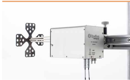
Model 7651 planar biaxial extensometer with tension-tension specimen
