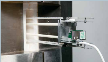
Self-supporting Model 3448 with clamshell-type materials testing furnace
