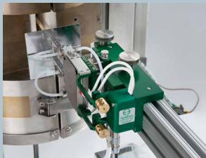
Model 3549 with 25 mm gauge length
