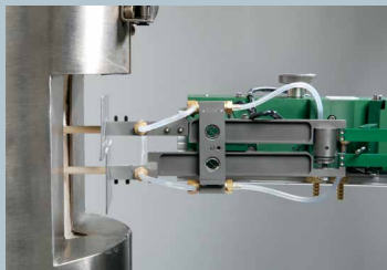
Model 3648 with 1 inch gauge length
