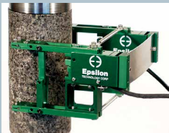
Model 3542RA1 extensometer with 50 mm gauge length
