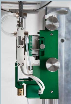
Model 3549 contact force scale for repeatable placement against test specimens
