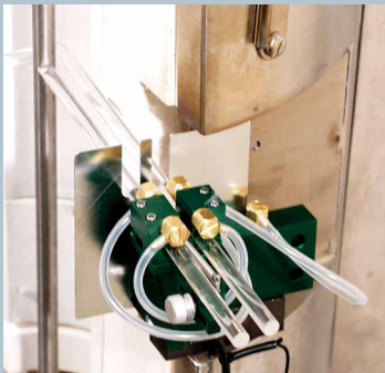
Model 3580 mounted to split furnace
