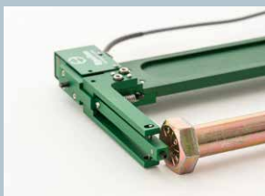
Mechanical overtravel protection for the upper arm and a break-away lower arm protect the extensometer if the bolt fails
