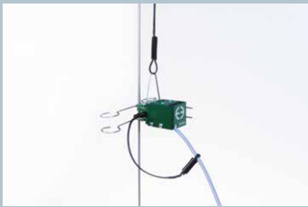
Model 3442 with 6.0 mm gauge length, ±1.0 mm (±16.7% strain) measuring range, and suspension tether
